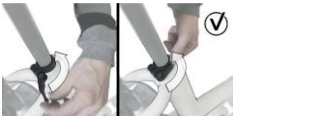
Image 8: Closing the seat post quick release
