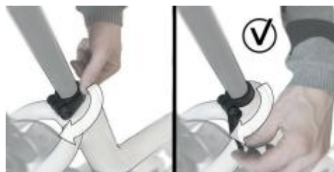
Image 6: Opening the seat post quick release
