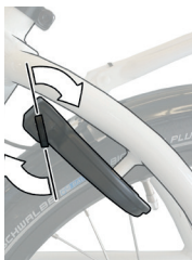
Image 29: Rotate the key 20 to 30 degrees clockwise
