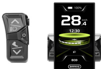
Image 21: Switching the display on and off
