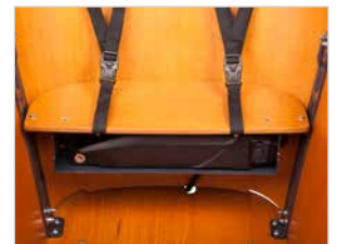
Battery underneath the bench
