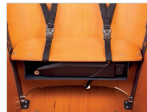
Battery underneath the bench
