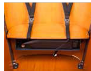
Battery underneath the bench
